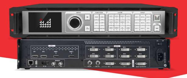
LED-EC40 Series product is video switcher developed for display system, using industry's top image processing chip, 24 bit digital processing, and 4K/60Hz 4: 4: 4 image processing technology. These makes image more clearer and colorful, built-in 4K and 2K matrix can support fade switch between multiple 4K and 2K inputs.
