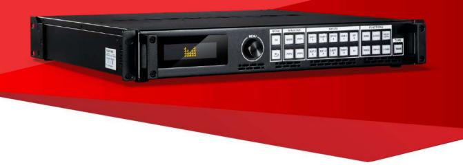
LED-750H, a superior approach to better visual performance for LED walls. It is a  $4K \times 1K/60Hz$  capable video processor. With EDID and customize output managment, it delievers high quality pixel-to pixel display via its user-friendly controls. It is an ideal choice for multi-media hall, multi-purpose room, theater, studio and showroom.
