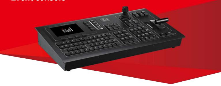
Single MIG-H2 event console can control 9 V2 at most, when works with V2 .itcan realize multidisplay effects, multi-layer switching, multi-scene switching, backup, etc. And it widely applied in auto show, conference, products launching, and stage show etc events.
