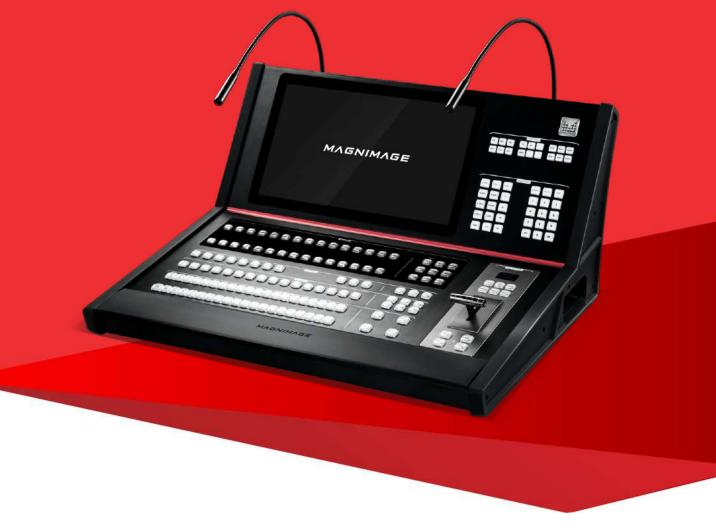
MIG-H6 is the latest Magnimage medium video console with a high performance CPU whose processing performance is very powerful. Equipped with one 18.5-inch HD touch screen, which can easily switch among inputs and outputs, setup layers, target scene and real time target presets monitoring seamlessly.
