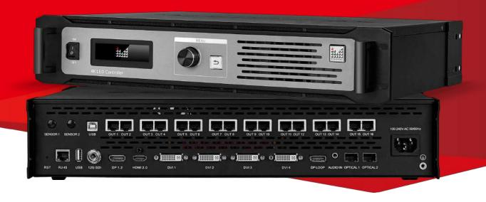
LED-T16S-A is a LED controller developed by Magnimage, input support 4x DVI, 1x DP1.2, 1x HDMI2.0, 1x 12G SDI(optional), 1x 3.5mm audio.Output support 16 x Gigabit Ethernet ports, 1x HDMI-Loop. Besides, it also supports 2 sensor interface, can be connected with external sensor, and expansion of 10G Optical fiber input / output.
