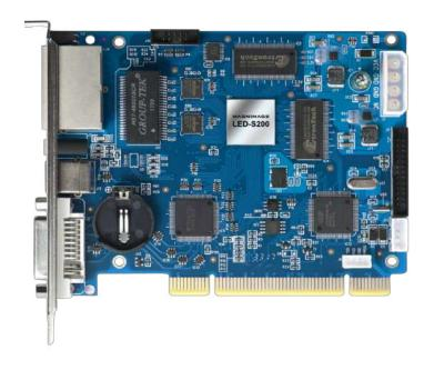
1--Communication light: Network port communication light. Green light flashing means normal communication, green light is always on means disconnected, red light is power indicator light, alwaus light means power supply is normal.
