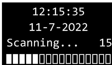
The device scans for all available DAB+ radio stations and it shows (in real-time) the number of found DAB+ radio stations. When a scan is complete, the device activates the first of the found radio stations:
