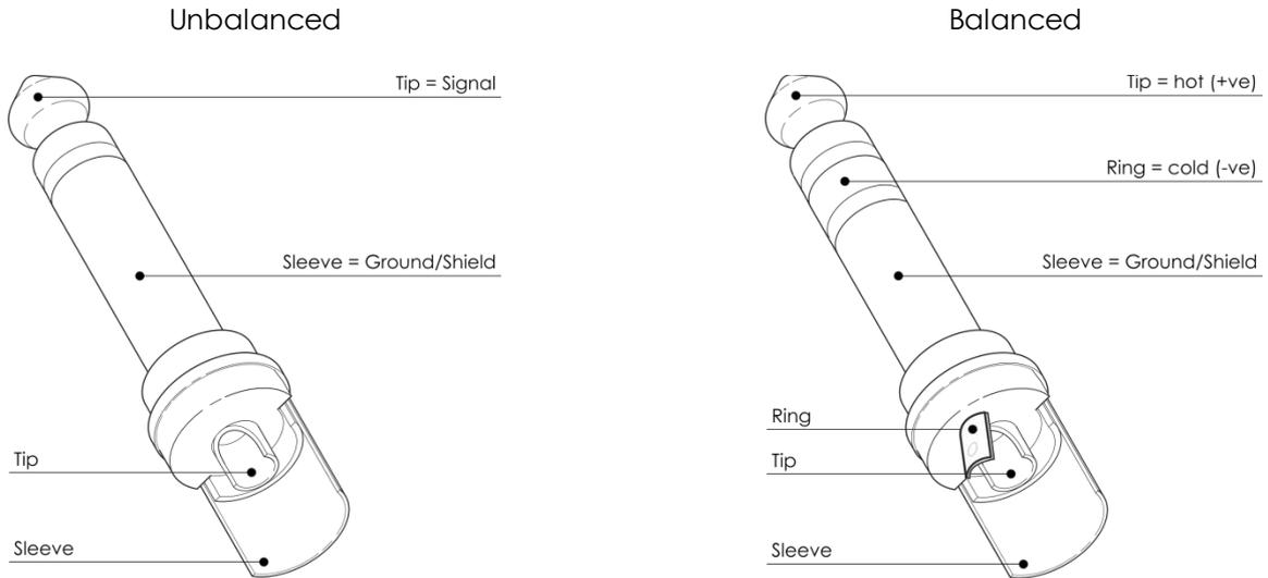
For these applications the unit provides 1/4" TRS and XLR connectors to easily interface with most professional audio devices. Follow the configuration examples below for your particular connection.
