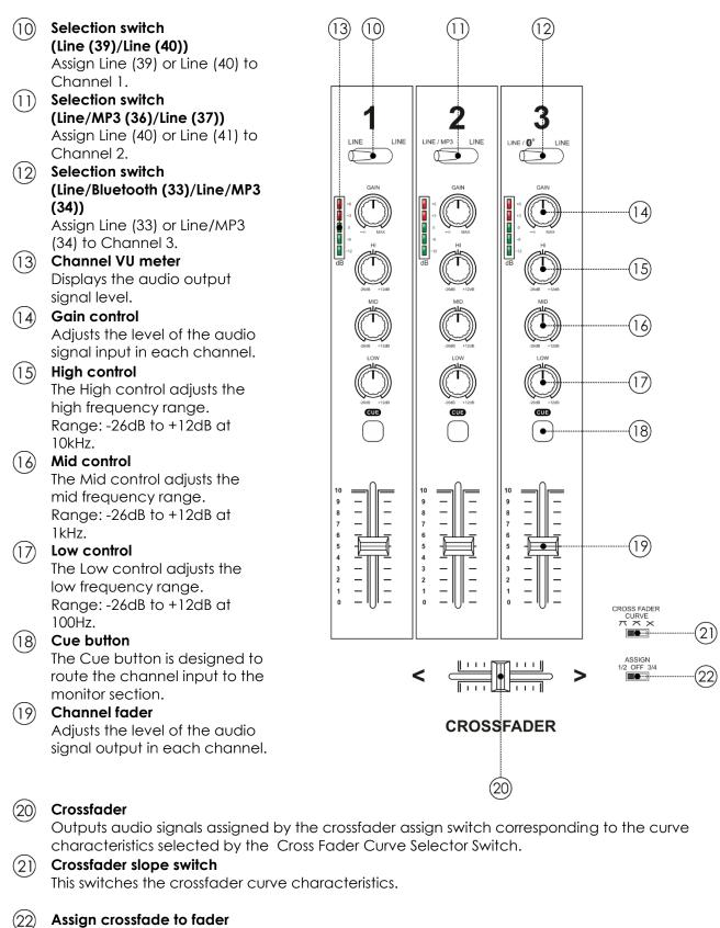
Assigns the channels 1/2 or 2/3 to the crossfader.
