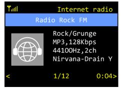
Press and hold down the **TUNE/SELECT** control for 5 seconds to save the internet radio station to My Favourite. The display promptly shows:
