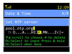
01) Turn the **TUNE/SELECT** control to choose characters and press the **TUNE/SELECT** control to confirm. Repeat this step to type in the address of the time server. The available characters are uppercase and lowercase letters, digits, punctuation marks, and some symbols.
