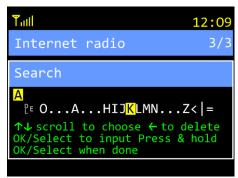
03) Turn the **TUNE/SELECT** control to choose characters and press the **TUNE/SELECT** control to confirm. Repeat this step to type in the desired word or phrase. The available characters are uppercase letters, digits, punctuation marks, and some symbols.
