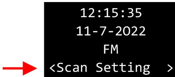
The settings menu is visible in the bottom line of the display.
