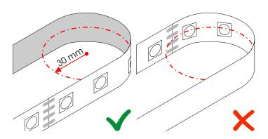
You can bend the LED strip only along the vertical axis. The maximum bending radius is 30 mm
