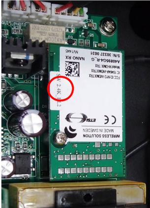
**The Part Number of Optional Wireless DMX module is W-DMX-PCBR (1 x W-DMX antenna + 1 x W-DMX board)**
