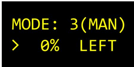
04) Press the **UP/DOWN** buttons to set rotation speed. The adjustment range is 0–100 %, from slow to fast.
