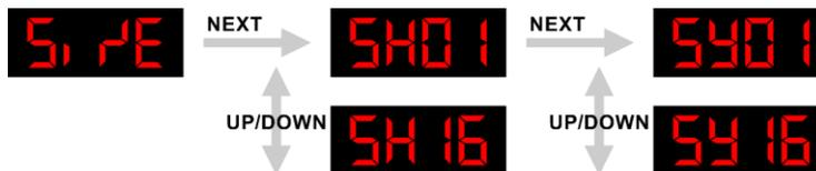
01) Press the **UP/DOWN ARROW** keys to adjust the width (X axis). The adjustment range is 01–16.
