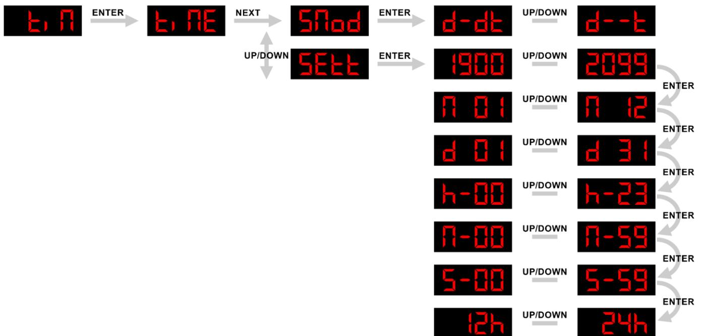
01) Press the **ENTER** key to activate time mode. The time is projected.
