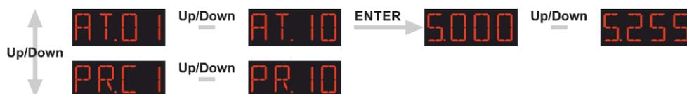
03) Press the **UP/DOWN** buttons to set the program speed. The adjustment range is between 0–255, from slow to fast.
