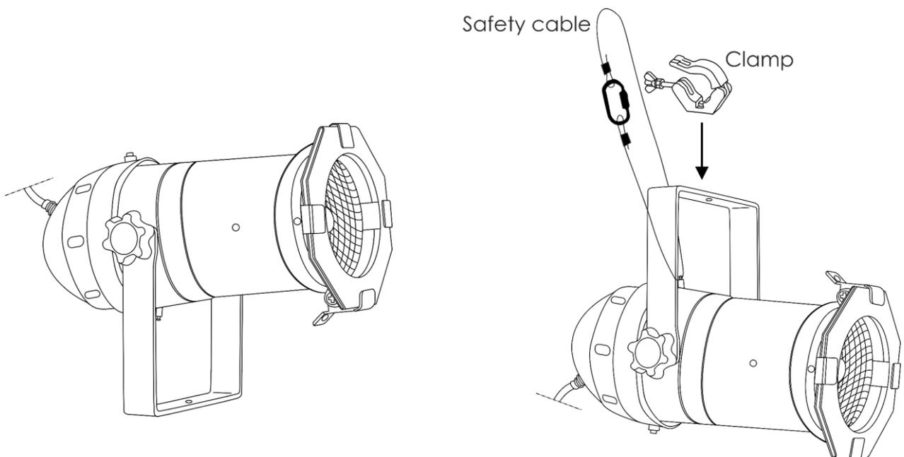
The PAR 46 Warm-On-Dim can be placed on a flat stage floor or mounted to any kind of truss by a clamp.
