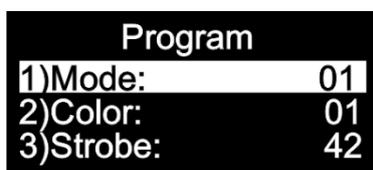
03) Press the **UP/DOWN** buttons to scroll through the built-in programs. The adjustment range is between
