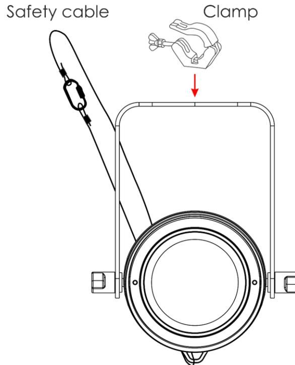
The Cameleon Spot Q4 can be placed on a flat stage floor or mounted to any kind of truss with a clamp.
