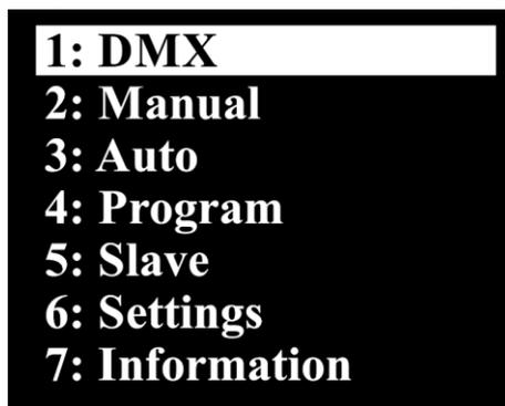
03) Press the **UP/DOWN** buttons to toggle between the menus.
