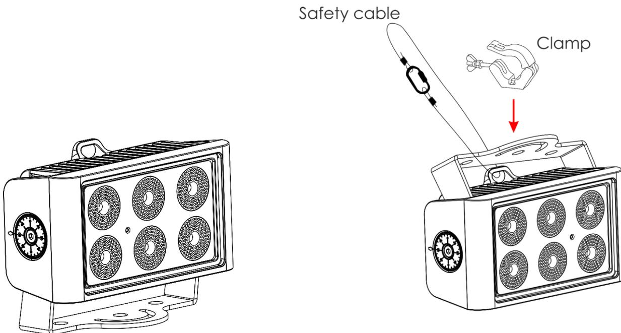
The Cameleon Flood 6 Q4 can be placed on a flat stage floor or mounted to any kind of truss with a clamp.
