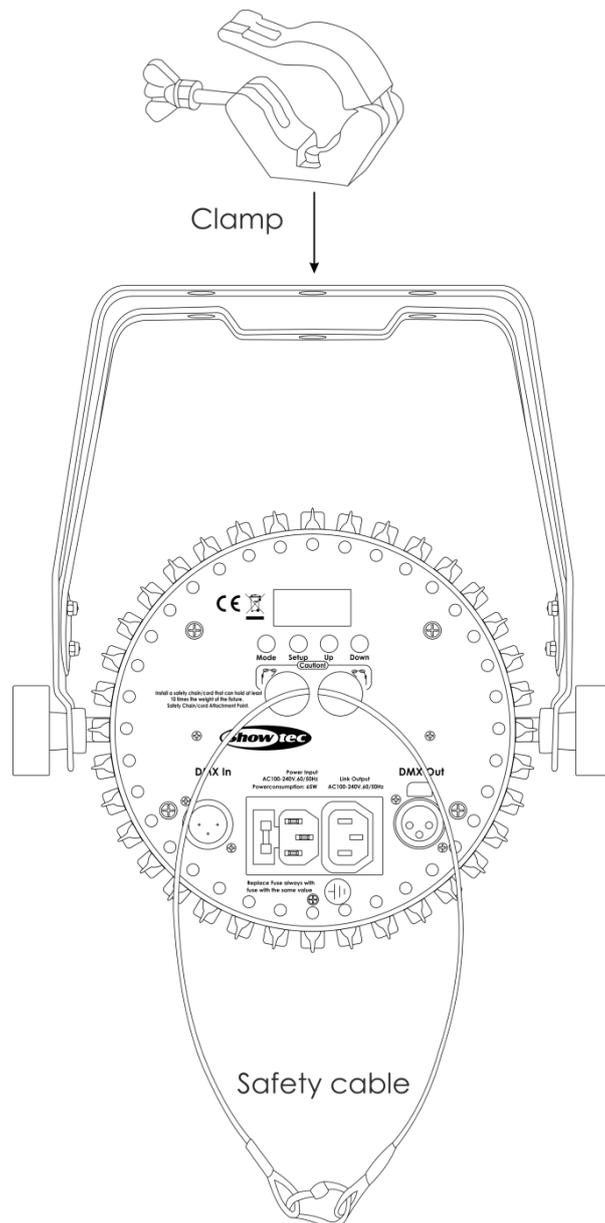
The Power Spot can be placed on a flat stage floor or mounted to any kind of truss with a clamp.
