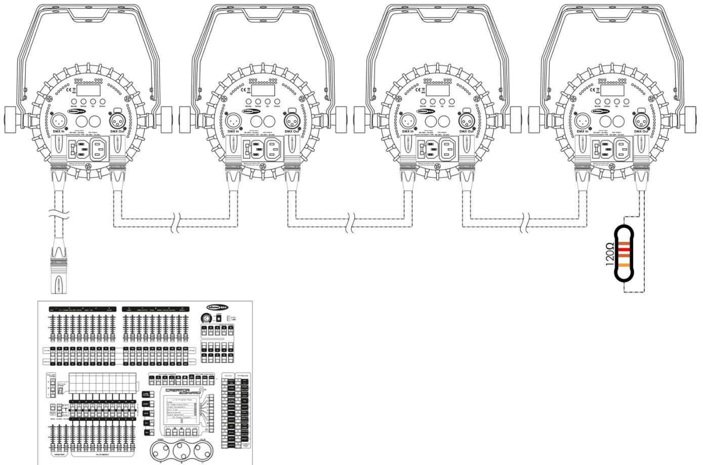
Note : Link all cables before connecting electric power
