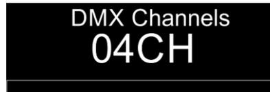
02) Press the **UP/DOWN** buttons to set the desired DMX channel mode. Choose one of the 5 options:
