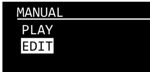
01) Press the **UP/DOWN** buttons to choose EDIT and press the **ENTER** button to open the menu. The display will show:
