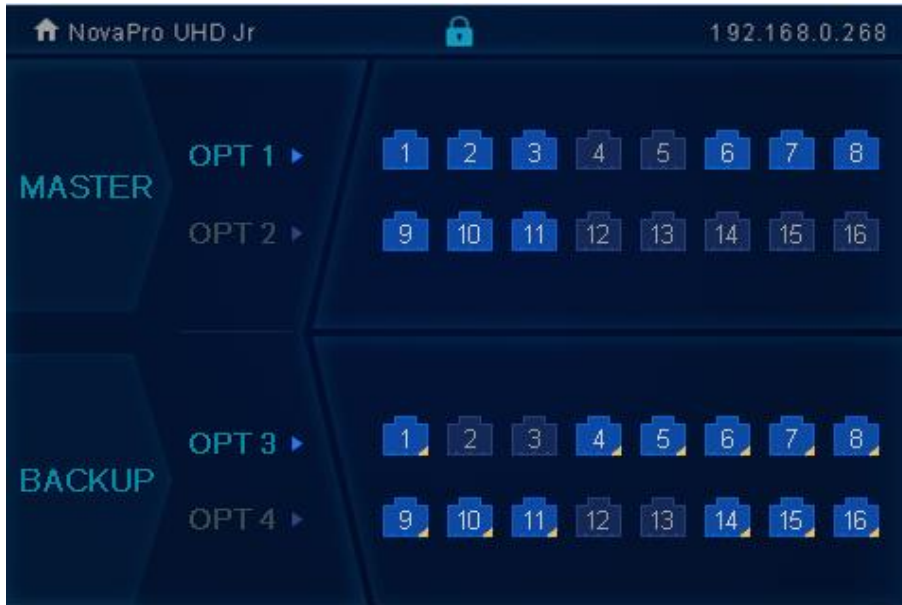
Figure 4-3 Optical fiber port statuses – Hot backup
