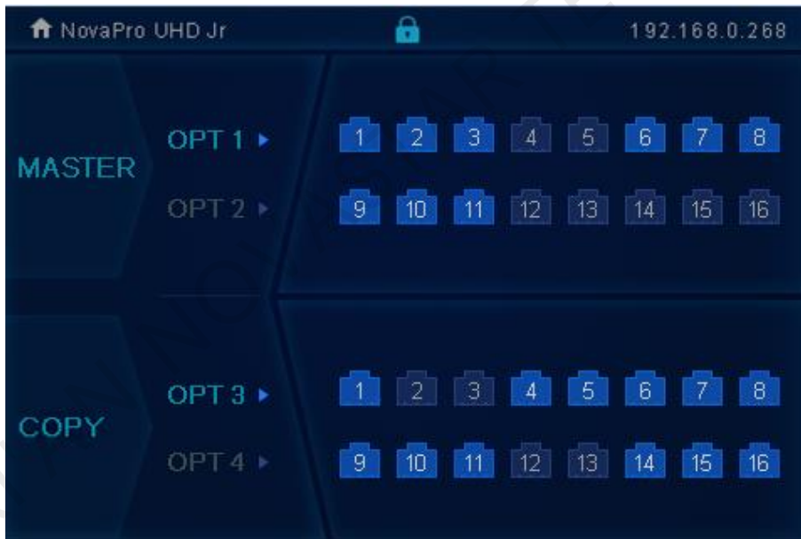
Figure 4-2 Optical fiber port statuses – Copy
