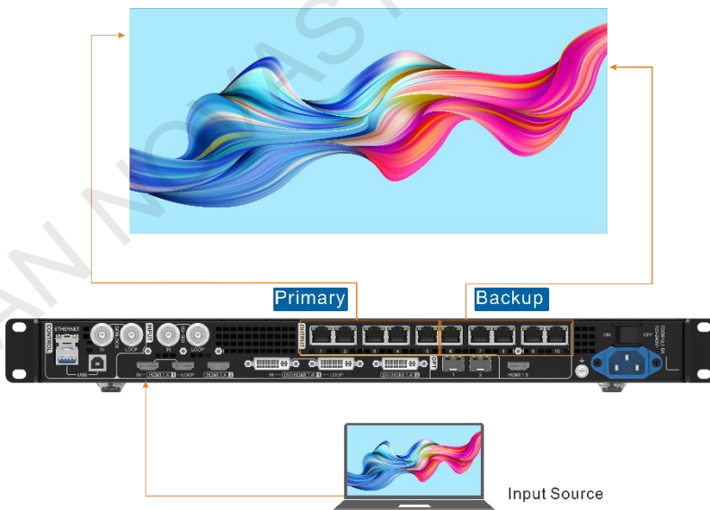
Figure 5-27 Ethernet port backup connection
